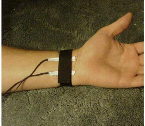
NOTE: BOTH ELECTRODES RUN PARALLEL ALONG THE RADIAL AND ULNAR ARTERIES
